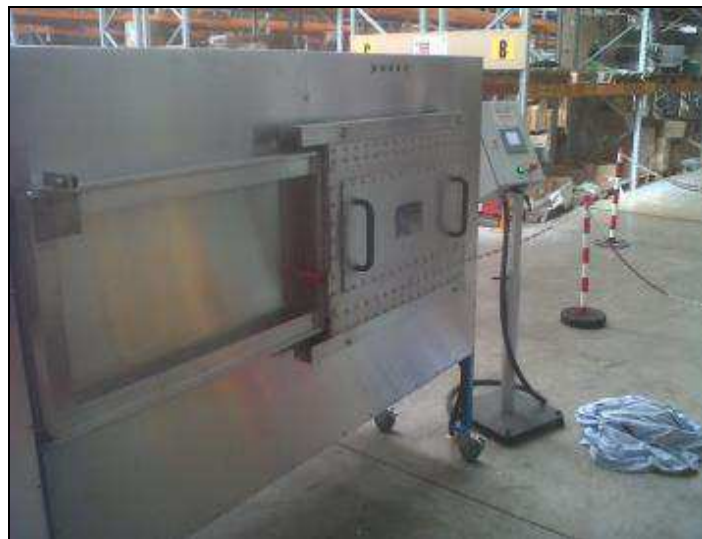
Figure 7: wear2 prototype microwave seam disassembly unit
