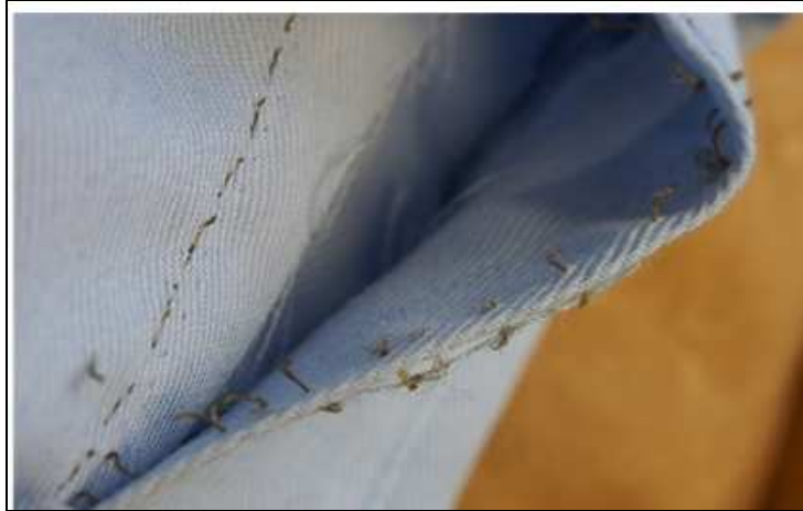
Figure 5: Seam separation after microwave processing, demonstrating yarn breakage at multiple points
