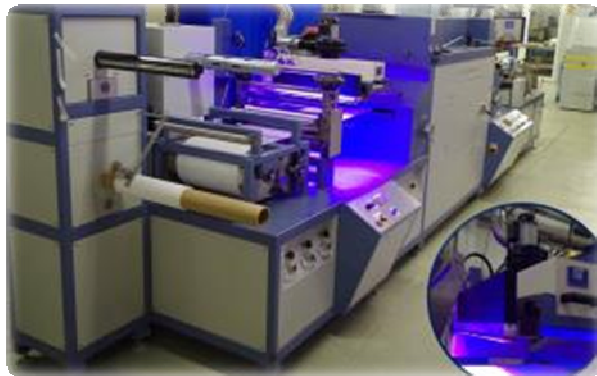
Figure 11: Lab-scale coating plant with integrated UV-LED aggregate (Photos: STFI)
