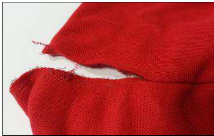
Figure 6: Seam separation after microwave processing, showing that fabric is undamaged
